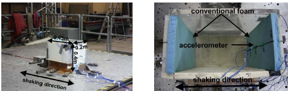
Figure 15. Rigid soil container with absorbing boundaries used at the Bristol Laboratory for Advanced Dynamics Engineering (BLADE). A soft material, namely conventional foam was applied at both end-walls of a small soil container (Lombardi and Bhattacharya, 2012).
